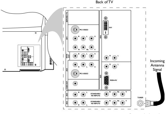
Connect the incoming Antenna signal to the TUNER jack on the back of the TV.
